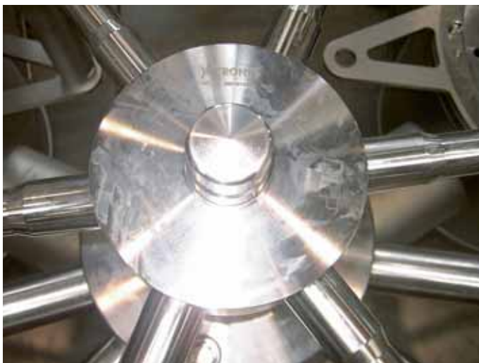
This ETP-EXPRESS R is made of high grade stainless steel, because it is washed regularly with an aggressive cleaning fluid.
