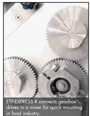
Easy adjustment of chains, relative to each other, and location of the sprockets, with ETP-EXPRESS R.
