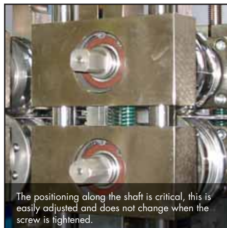
Rollers are easily changed using ETP-POWER and especially beneficial in high production applications.
