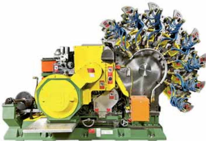
This customized ETP-AXPRESS fastens and centers the decorating cylinder for printing on the outside of beverage cans.
