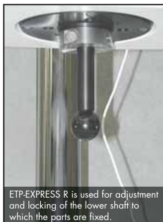
Easy adjustment of chains, relative to each other, and location of the sprockets, with ETP-EXPRESS R.
